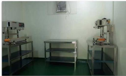
Gambar 17. Mesin Cotinuous Sealer
