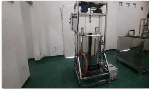
**Gambar 12.** Mesin Pasteurizer Kapasitas 50 Liter
