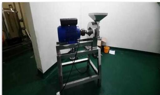
**Gambar 15.** Mesin hammer mill
